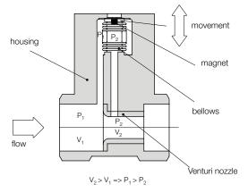
If the flow is exceeded the differential pressure measuring cell is protected by locking pins. On mechanical displays the flow rate measured by the pressure measuring cell is transferred via a pointer movement to the pointer indicator calibrated in I/min water or Nm<sup>3</sup>/h air. On electronic displays the mechanical motion is converted to an electrical signal by a Hall-sensor. Various electronic modules are then used to display and monitor the volumetric flow.
