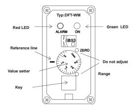
Attention! When the red light emitting diode is flashing the limit value relay is in alarm condition (see connection diagram).
