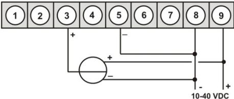
**ADI-1V -devices with current input / voltage input and sensor supply**
