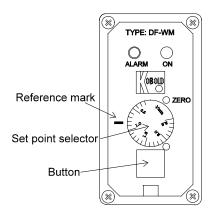
The instrument is delivered ready to operate. The electronics are matched and calibrated with the signal transmitter. The calibration screws ('ZERO' and 'RANGE') next to the rotating scale adjustment knob must not be adjusted by the customer. If they are adjusted, a re-calibration will be required involving new calculations. Should the electronics be opened, any warranty will become invalid. As soon as the external power supply to the instrument is switched on, a green LED will indicate that
